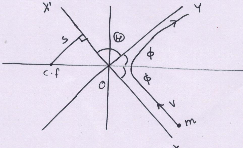
The angle  $x'oy = \Theta$  is called angle of scattering & perpendicular distance ( $s$ ) is called the impact parameter.
