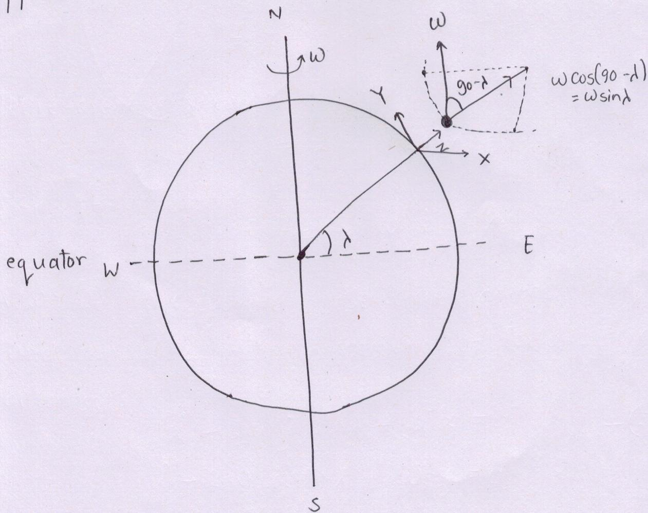
At an  $\alpha$  latitude  $\lambda$ , the angular velocity ( $\omega$ ) can be resolved into two components  $\omega \sin \lambda$  and horizontal component  $\omega \cos \lambda$  in N-S direction.
